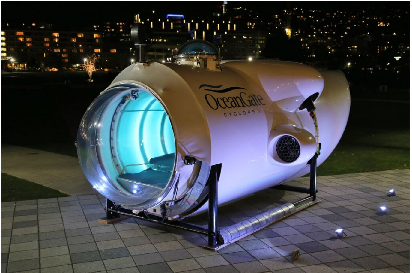
OceanGate's Cyclops 1, the predecessor of the Titan sub. The Titan had a 380 mm (15 inch) window.
